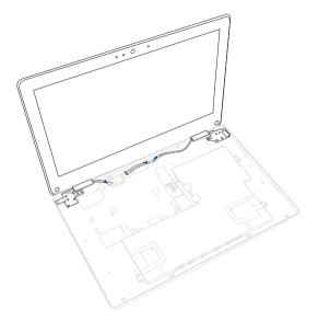
D. Remove the screw(s) from the hinges, and then remove the LCD panel module.
