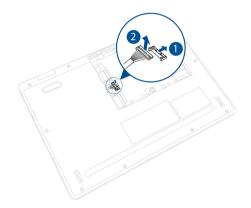
To connect the battery, align and connect the cable to the battery connector before you reattach the compartment cover.
