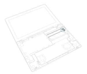
J. Reattach the mylar to secure the USB board.
